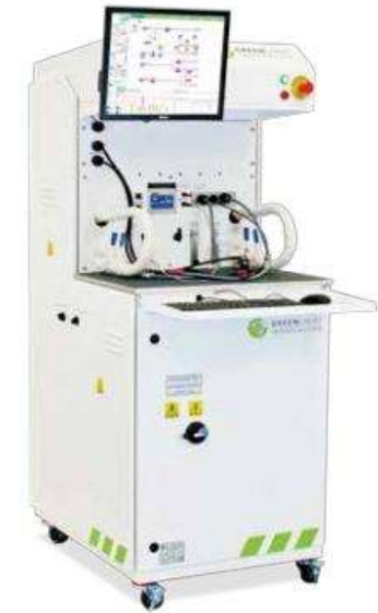
A Greenlight Fuel Cell Test Station (G40 Fuel Cell System, Hydrogenics, Canada)
