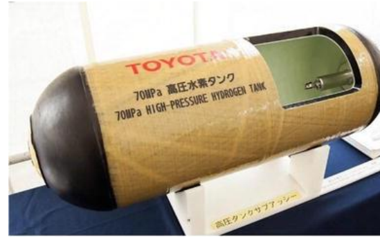
Type IV H 2 tank for 700 bar (left) and 60 bar (right) storage
